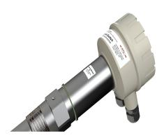
To protect the electronics from too high temperatures, a temperature insulating tube gets mounted in between the process connection and the enclosure. Instead it is as well possible to install the electronics at a place with lower ambient temperature by using the remote electronics installation.
